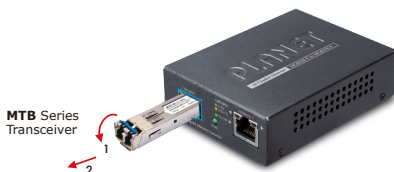
Figure 3-5-2: Pulling Out from the Transceiver
