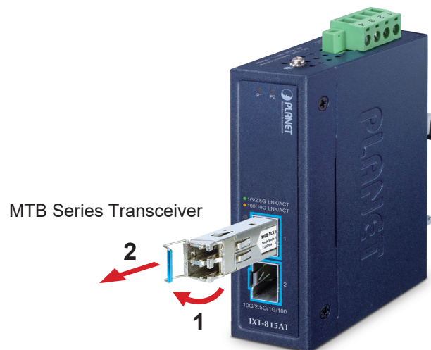
Figure 5-2: Pulling Out from the SFP+ Transceiver
