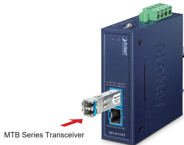
Figure 5-1: Plug in the SFP+ Transceiver
